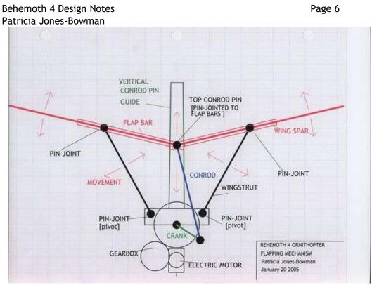
Fig 8 Flapping Mechanism
