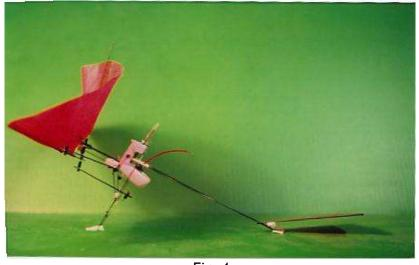
Fig 4 Fuselage in maximum pitch down position
