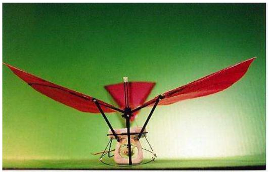
Fig 6 Wings at top of upstroke
