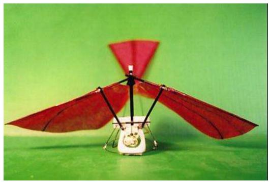
Fig 7 Wings at bottom of downstroke
